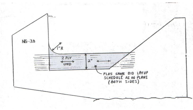
and additional 2 plies of BID, both sides, be added. Make this change in Chapter 13, page 2, Step 2, and on drawing M-10.
