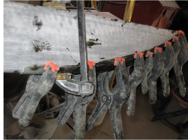
Liquid urethane rubber poured into a leading edge mold and clamped into position until cured
