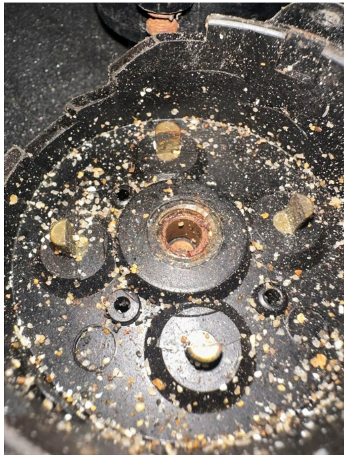
Figure 6: Second distributor cap - worn, but more serviceable contacts
