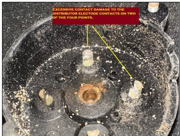
Figure 3: Distributor contact damage
