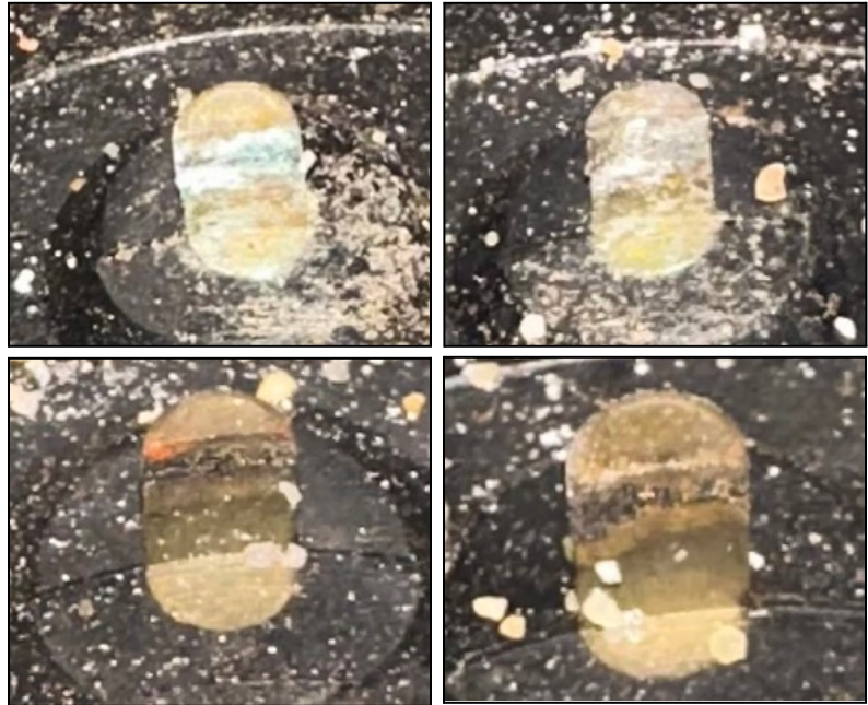
Figure 4: Closeup of distributor contact damage
