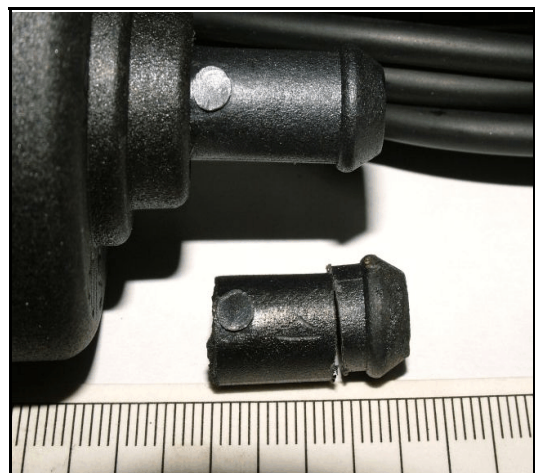
Figure 5: Recovered Inlet Post of Fuel Flow Transducer compared to Exemplar
