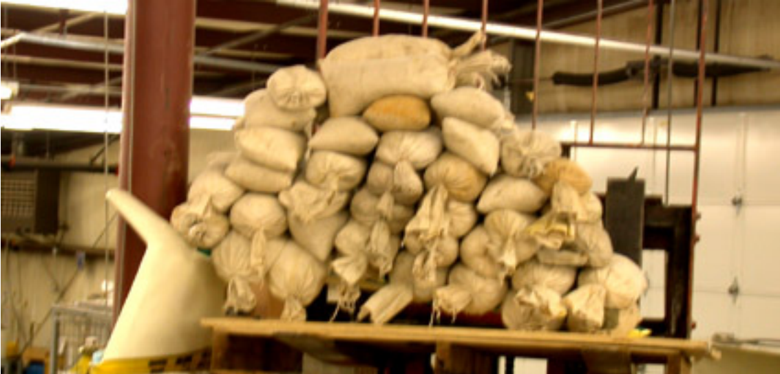
The steel support post & top of the wing can be seen. There are 42 shot-bags on the outboard side of the winglet, and a forklift with a pallet on its forks, is positioned just under, but not touching in case of a failure. It did NOT fail, although this load was more than two times the required strength!
