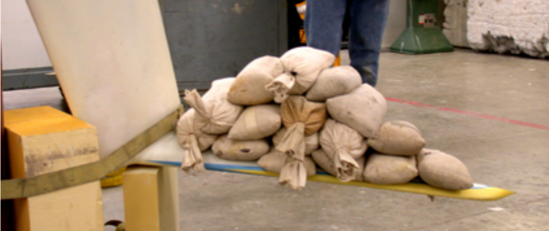
The wingtip is supported at the winglet root, and the shot-bags shown here represent design limit load. The winglet failed right at ultimate load.
