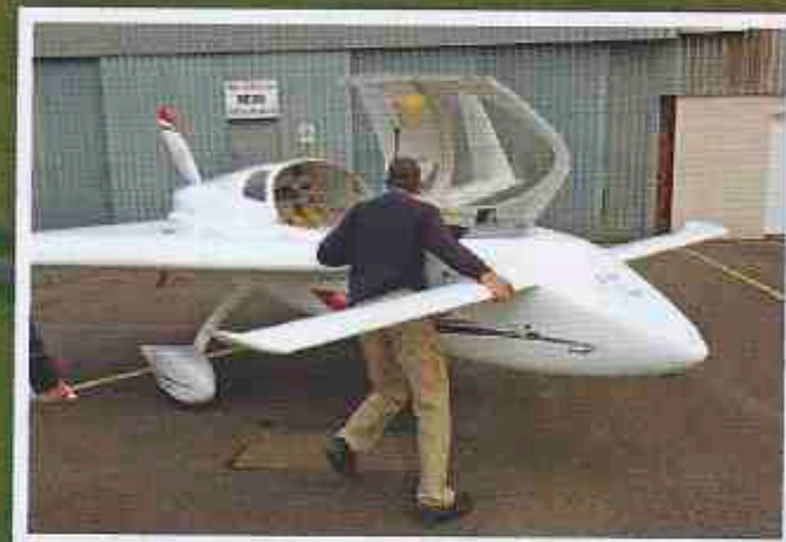
Moving the Cozy, as with the other Rutan-esque designs, requires the canard to be grasped for ground manoeuvring. Due to the C of G position without front seat passengers, they will tip backwards with undesirable consequences
